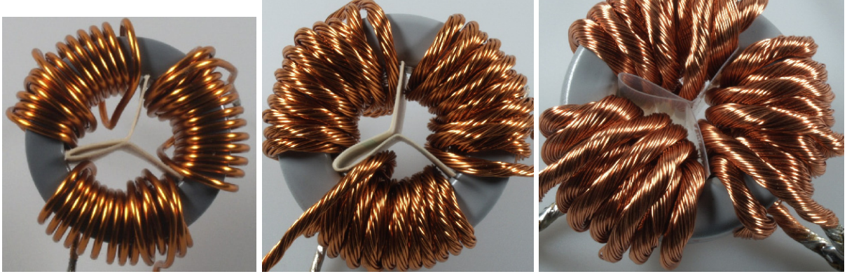
Fig. 2: A 2.2mH choke with massive wire for 10A, a 2.4mH with Litzwire for 18A and a multi-layered choke with 0.85mH for 25A
